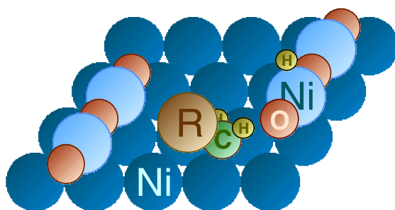
Figure 5. A schematic representation of the proposed catalytic site required for the partial oxidation of alkanes and alcohols. In this model, the oxygen atoms at the end of –Ni–O– rows are responsible for hydrocarbon conversion, interacting via hydrogen-bonding with the reactant alkyl species bonded to adjacent nickel atoms. Nearby hydroxide surface species are also required to enhance the oxygen insertion that leads to alkoxide formation, the first step in the oxidation process. The use of defective oxides with large numbers of partially oxidized nickel atoms, electronically unsaturated oxygen atoms, and neighbouring OH groups, all appear to be required for the selective oxidation of alkanes or alcohols towards aldehyde or ketone production.
